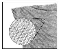
Pure 100% surgical stainless Steel (AISI316L), .004 inch diameter, knitted into a shielding fabric that's as strong as steel! Tight knit pattern yields good shielding. 26 dB at 800 MHz, 15 dB at 1900 MHz. Permits good air flow and light
